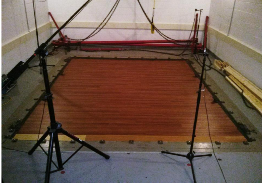
Source Room View of Test Specimen Installation
