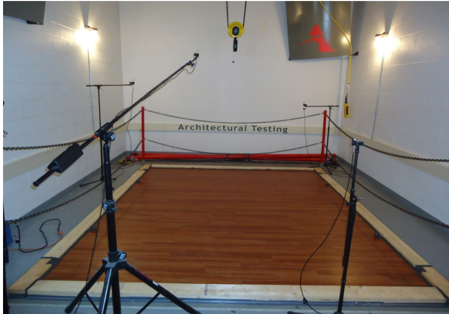
Source Room View of Test Specimen Installation
