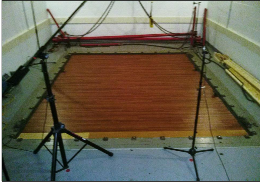
Source Room View of Test Specimen Installation
