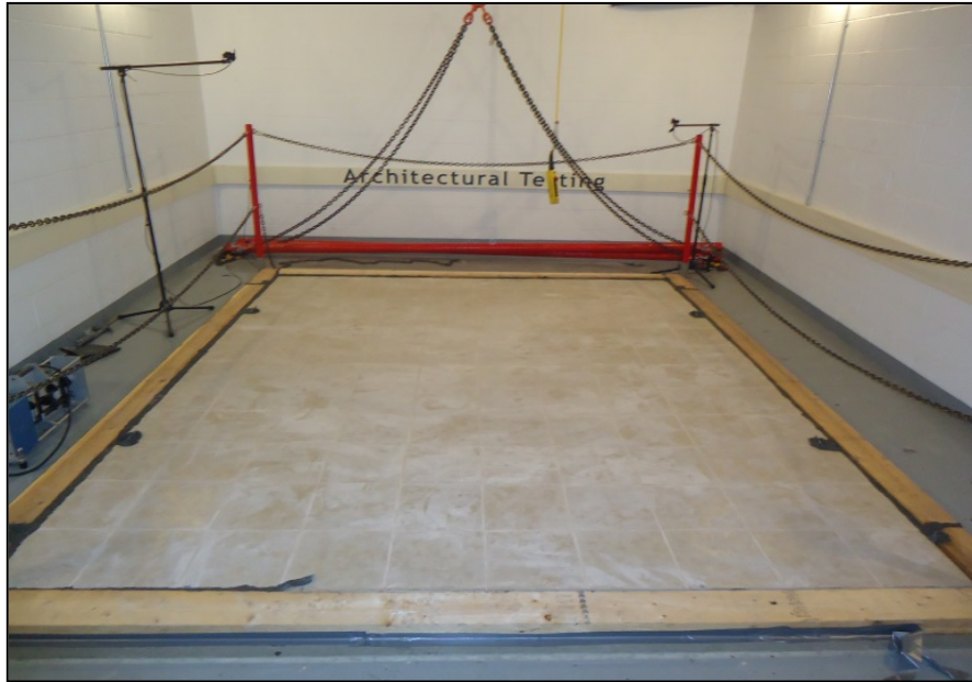
Source Room View of Test Specimen Installation
