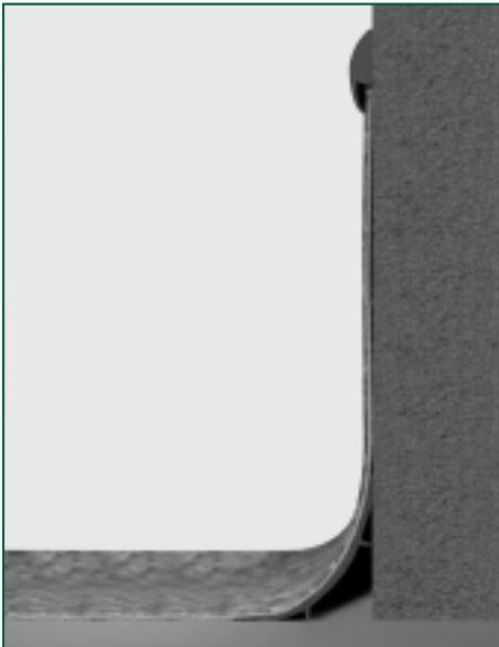
Figure 8 CS capping strip
