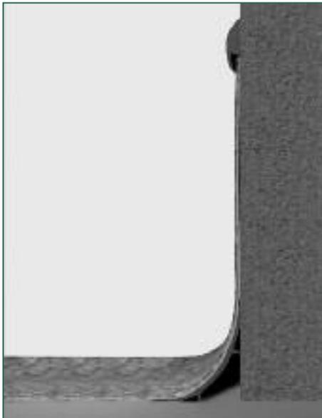
Figure 8 CS capping strip
