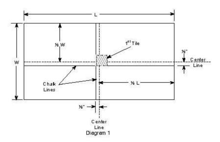
H. Interlocking tiles must be installed in the same direction. Directional markings stamped on the bottom of the tiles must point in the same direction. It may be necessary to offset the centerline to ensure that perimeter tiles are no less than 12".
