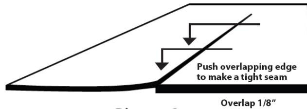
7. It may be necessary to trim the edge of the second lineal drop if the rolls do not extend the length or width of the room. Rolls laid end to end with a variance in roll width greater than 1/4" could result in peaked seams.
